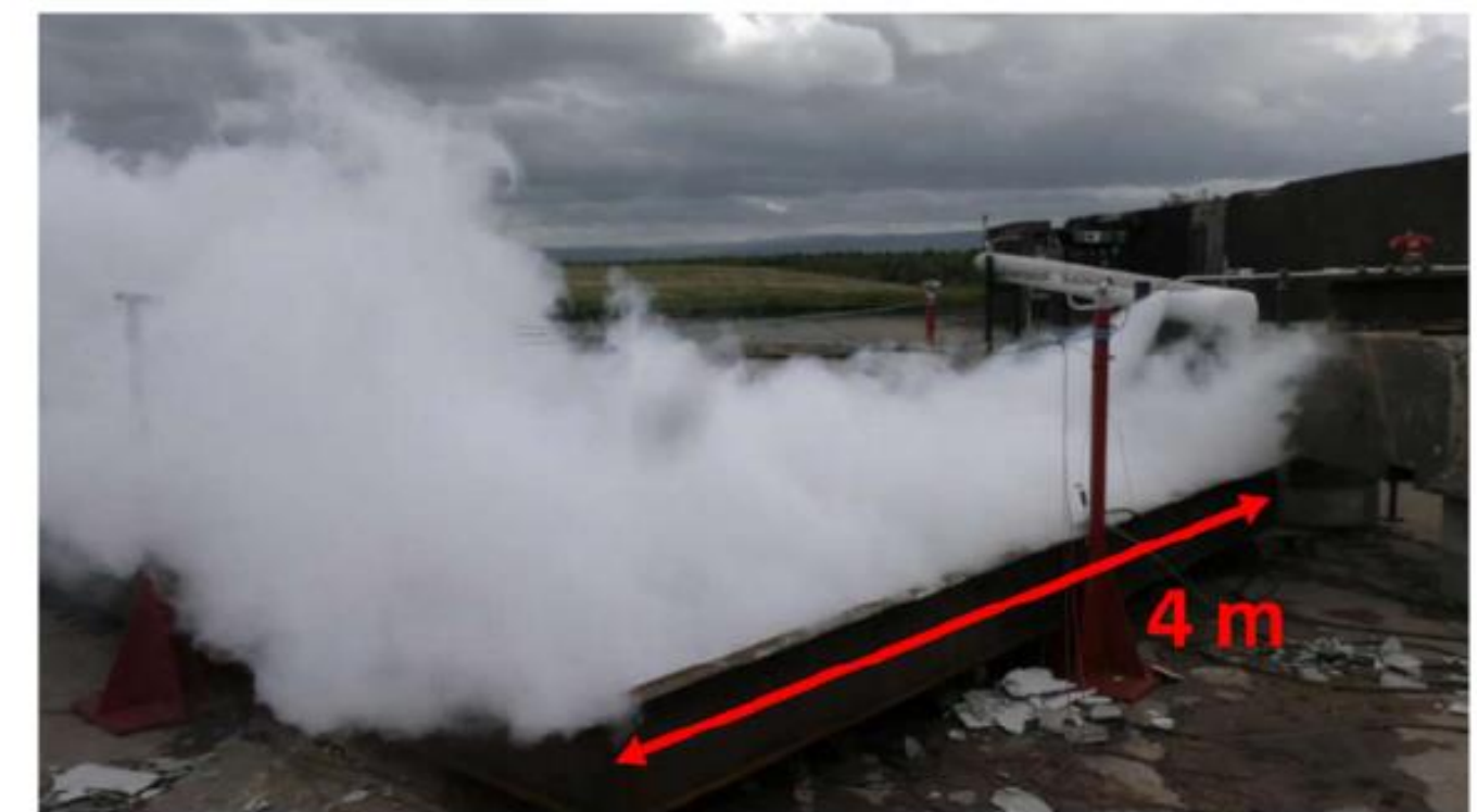
Figure 11: RS-3F refrigerated, pressurized ammonia release
